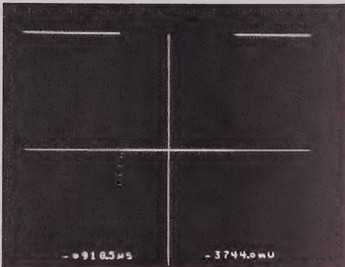
Figure 6 - Negative square wave cycle with undershoot.
